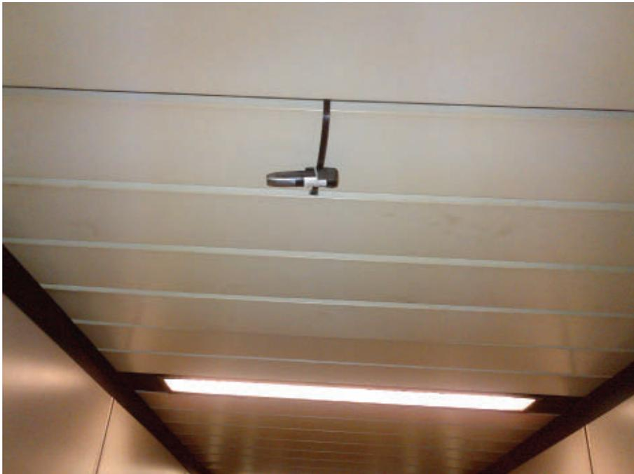
Dry bulb thermometer inside the bridge
