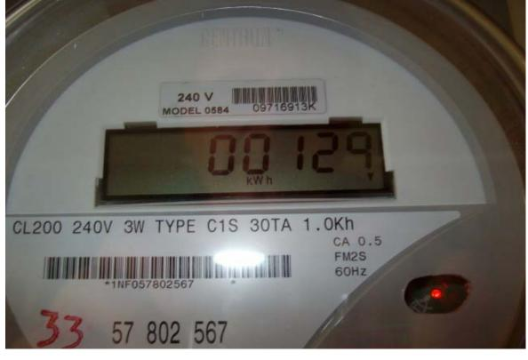
Figure 13 THIRD READING COATED ROOM 7/14/09 12:12 PM 129 KWH
